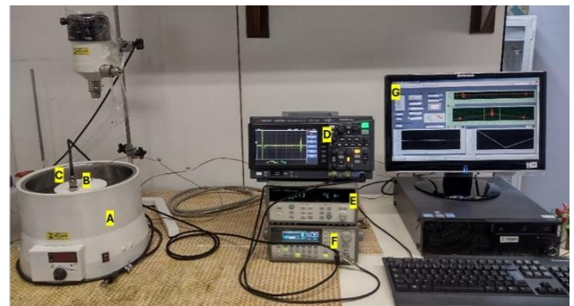
Figure 3. Characterization of the speed of sound of the analysed materials. A: thermal-controlled water bath; B: sample; C: transducer; D: oscilloscope; E: temperature measurement system; F: signal generator; G: software
