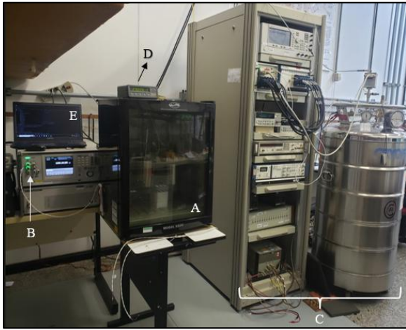
Figure 9. Setup of the electric current primary standard based on the PJVS and the QHS systems.
