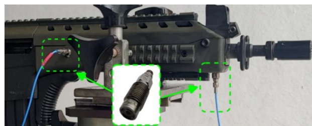
Figure 1. HPI GP6 piezoelectric transducer: instrumentation of a rifle using two units for chamber and muzzle pressure measurement.
