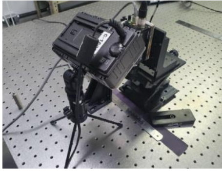
Figure 1. Experimental setup for capturing images of the scale.
