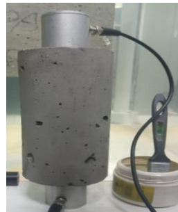
Figure 2 - Measurement of the specimen to obtain the ultrasonic velocity.
