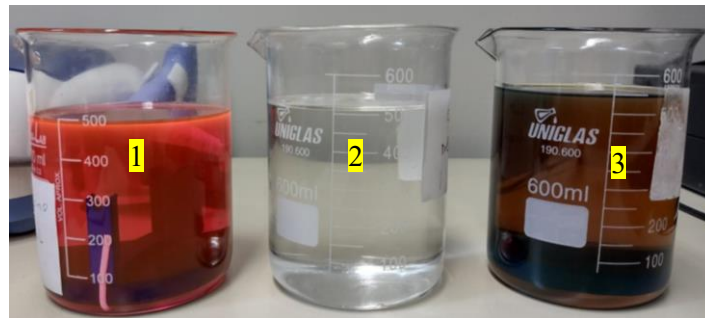
Figure 2. Samples used. (1) Ethylene glycol, (2) mineral oil, and (3) lubricating oil.
