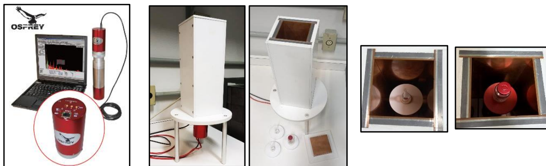
Figure 1- Arrangement of the gamma spectrometry system with NaI(Tl), assembled for characterization.
