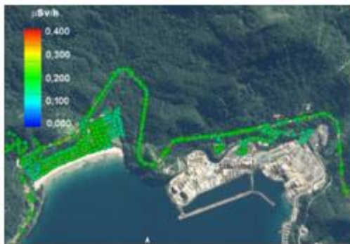
Figure 7 - Commercial Device Readings obtained: 3.33 nSv/min (average)
