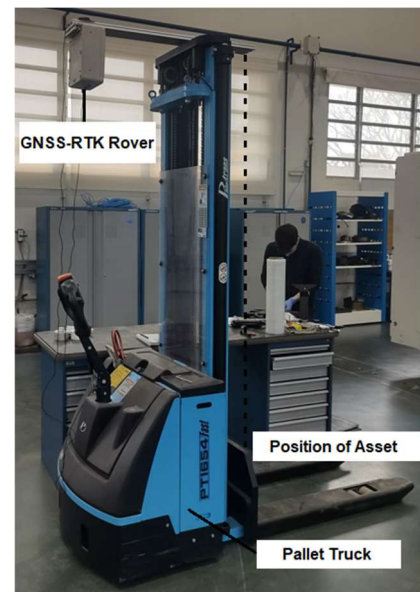
Figure 4. Installation of the GNSS-RTK rover on the pallet truck.
