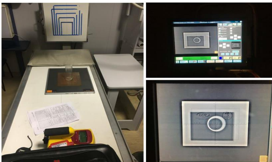
Figure 3 – Collimation test and central axis alignment.
