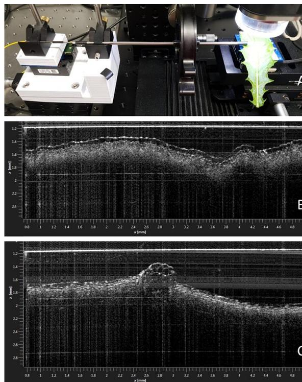
**Figure 6.** A) The probe prototype in the test fixture with a *T. officinale* leaf (front being measured). B) Front side measurement C) Back side measurement with central vein.
