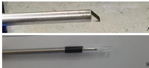
**Figure 5.** A) the FLP assembly with the prism showing B) the completed probe prototype with the FLP inside the metal sheath and quartz cap.
