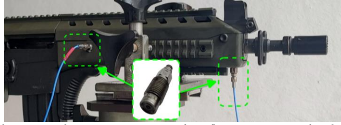
Fig. 3: HPI GP6 piezoelectric transducer: instrumentation of a rifle using two units for chamber and muzzle pressure measurement.
