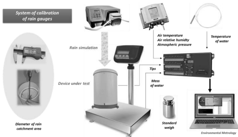
Figure 1 – Setup of calibration of rain gauge
