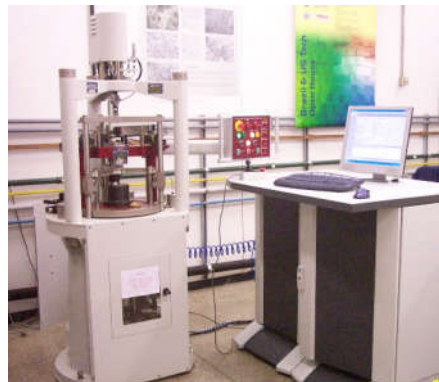
Figure 2. Inmetro's Hardness Primary Standardization Machine.
